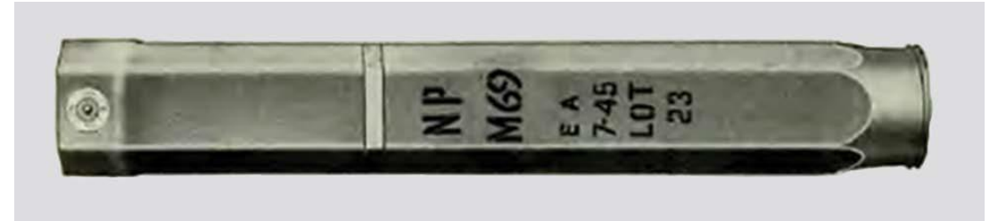
The E1, Bomb, Incendiary, Oil, 6 lb, M69. The bomb body was a hexagonal case with a nose cup welded to the forward end. The nose cup, fuze and powder charges were sealed off from the rest of the case by an impact diaphragm. The tail consists of gauze streamers about 4.5-inches in length.
