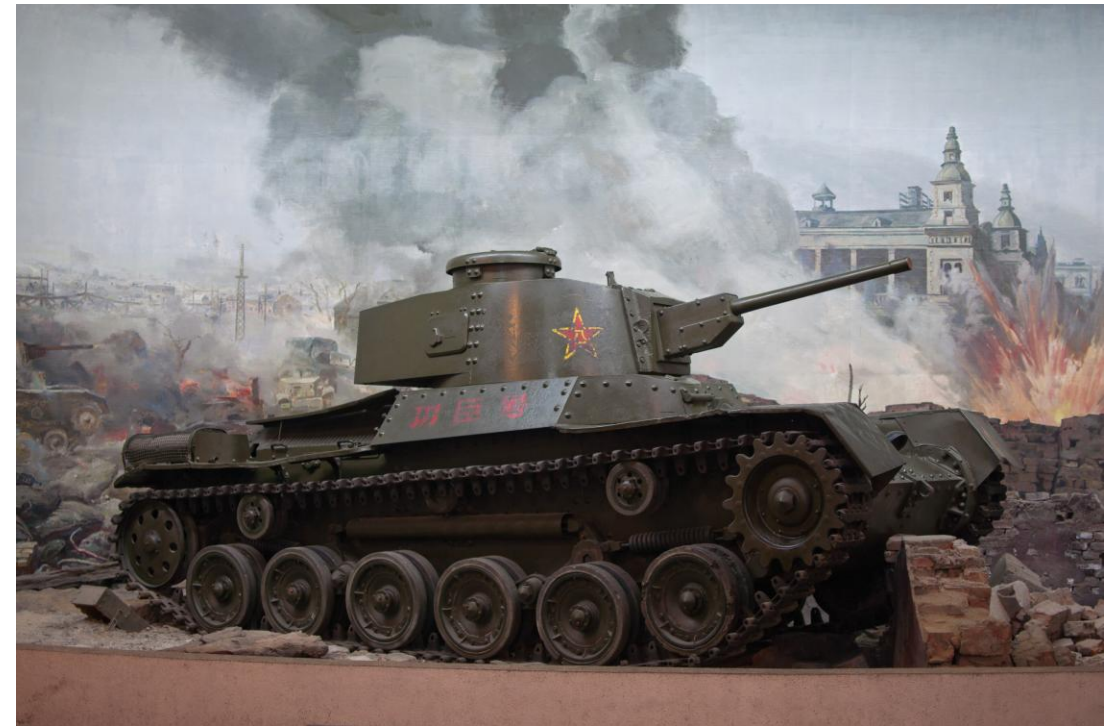
Type 97 Shinhōtō Chi-Ha "Gongchen tank" at the Beijing military museum. Crew of 5 (Commander, gunner, loader, bow gunner, driver) 1 x Type 1 47 mm tank gun 2 x 7.7 mm Type 97 machine gun. Front hull armor 25mm.
