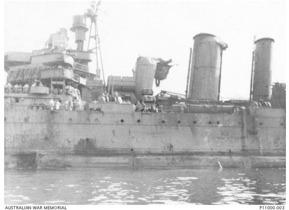
A view of the port side of HMAS Australia showing the hull damage inflicted by a Japanese Kamikaze attack on 8 January 1945.
