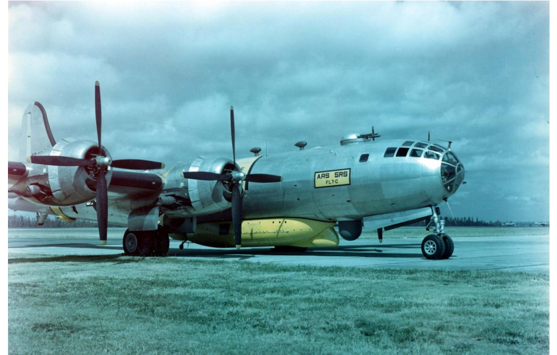
Boeing SB-29 "Super Dumbo" with AN/APQ-13 radome between the nose landing gear and the airborne lifeboat
