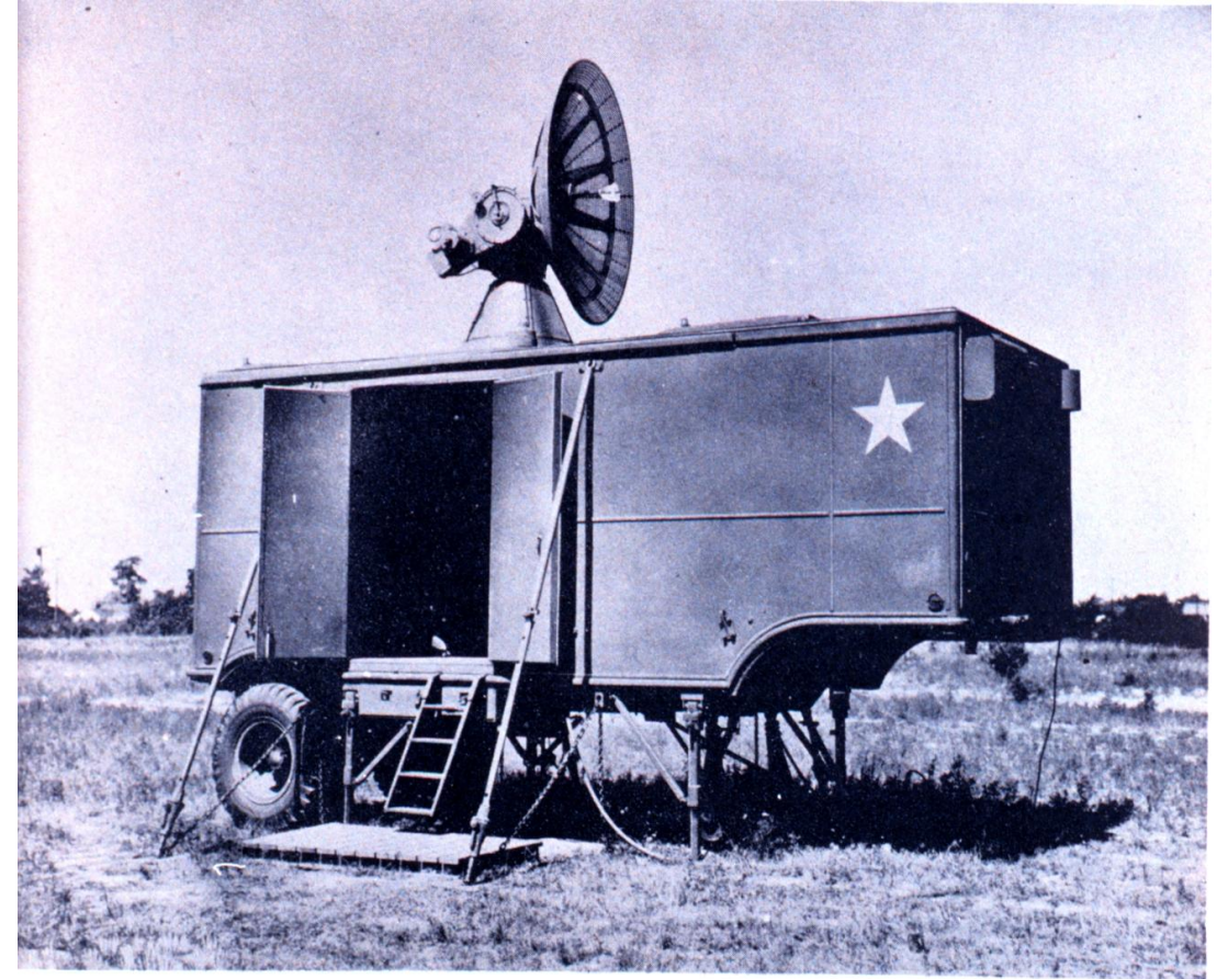
Figure 22. Exterior View of Radio Set SCR-584.
