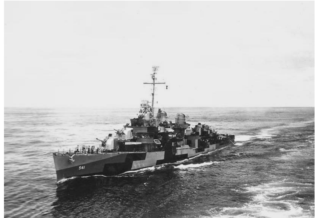
USS Yarnall underway in 1944. Laid down 5 December 1942. Commissioned 30 December 1943. 35 knots, 5 * 5 inch and 5 twin 40mm guns.
