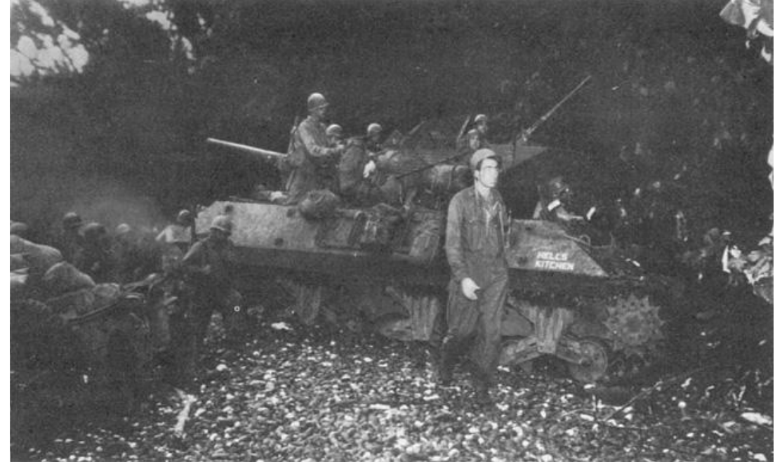
M 10 MOTOR CARRIAGE MOUNTING 3-INCH GUN on a rough and stony beach near Saidor, 2 January 1944.
