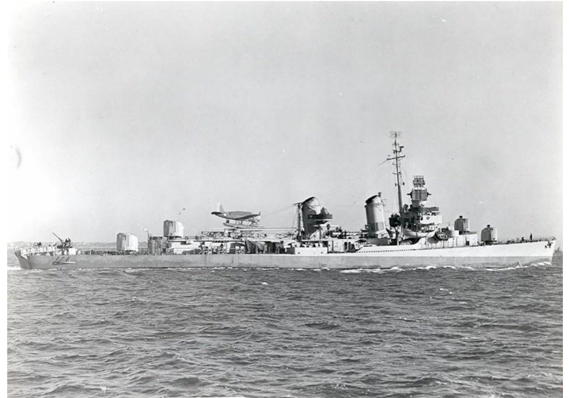
The U.S. Navy destroyer USS Pringle (DD-477) underway sometime in December 1942, location unknown. Note that she is fitted with a catapult and derrick, these were removed before her Pacific service. Note that the forward turrets have their top hatches open.
