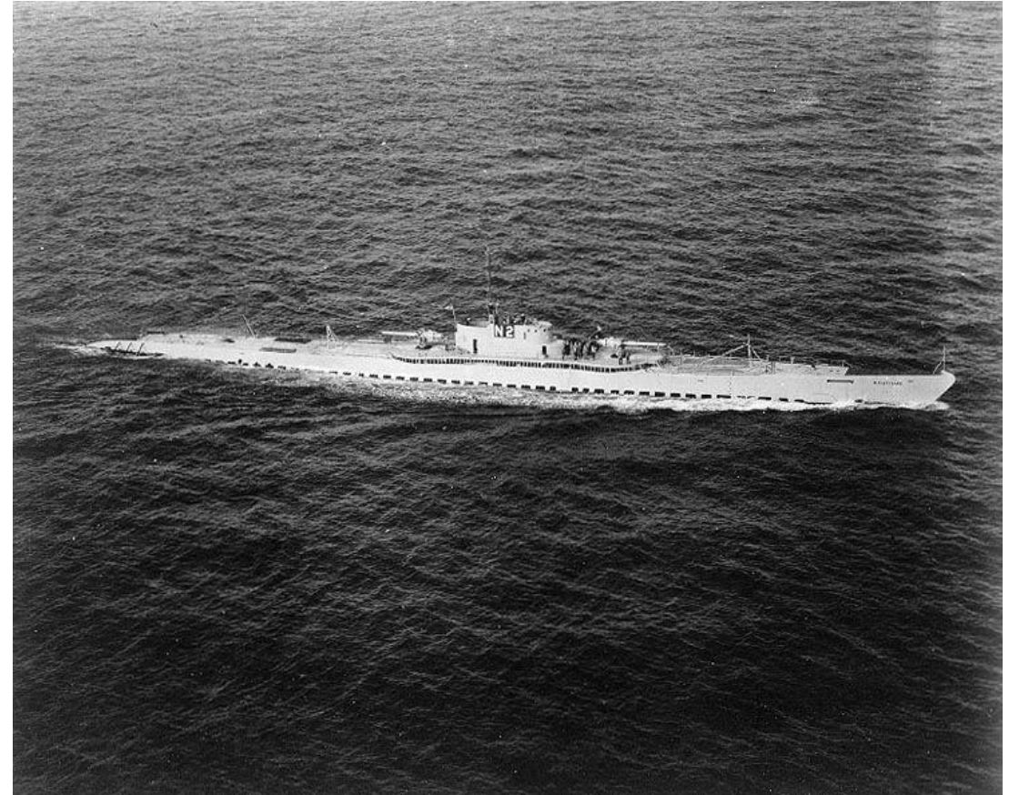
The U.S. Navy submarine N2 USS Nautilus (SS-168) underway in the early 1930s. 350 ft and displacing 4,000 tons submerged.
