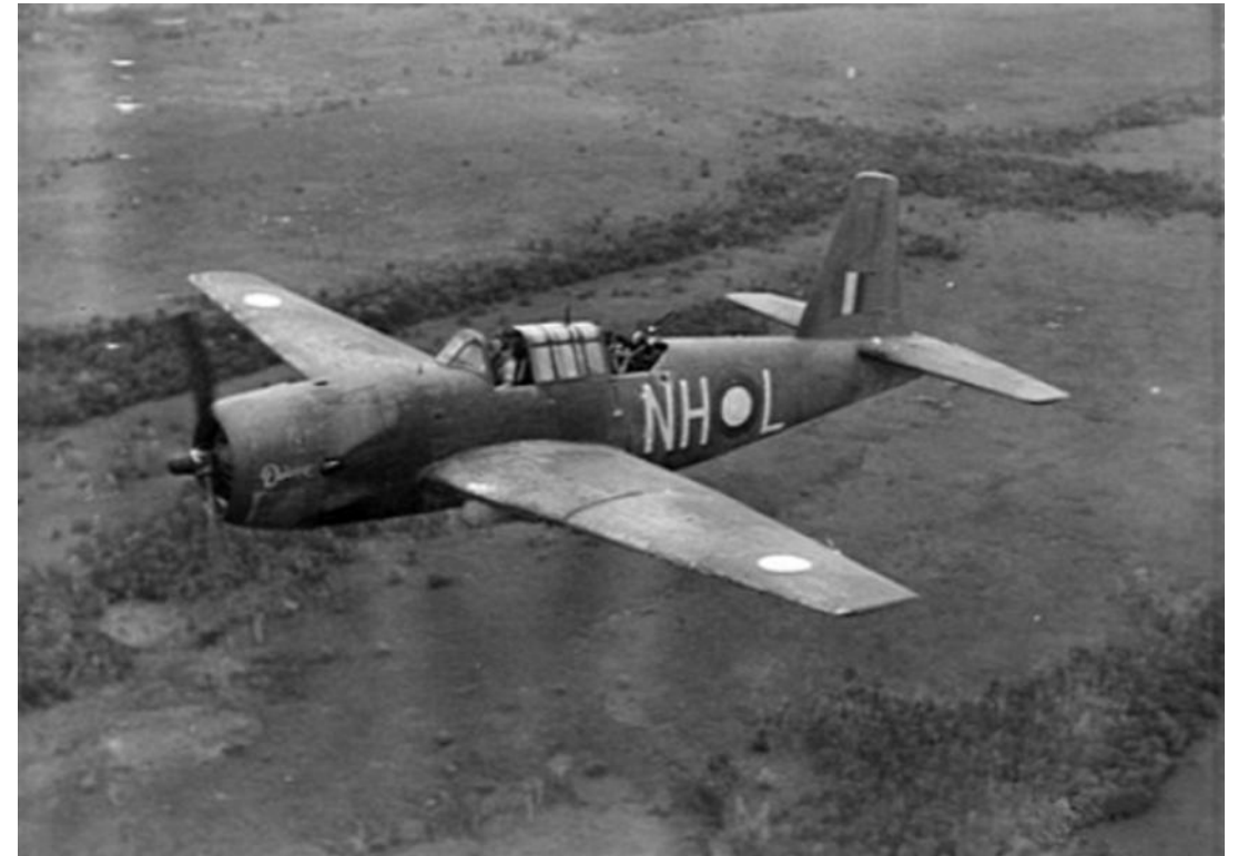
A Vultee Vengeance dive bomber, Max speed 275 mph, ceiling 22,500 ft, bomb load 1,500 lbs.
