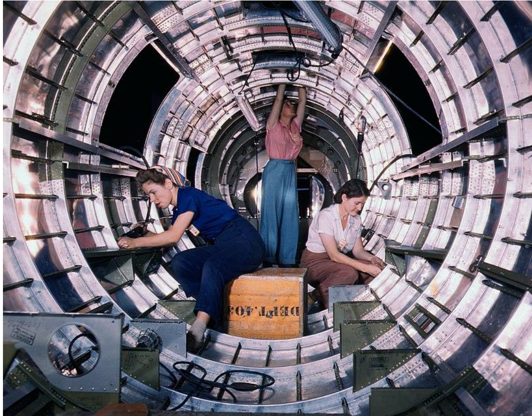
Installation of fixtures and assemblies on a tail fuselage section of a Boeing B-17 at the Douglas plant in Long Beach, California, October 1942
