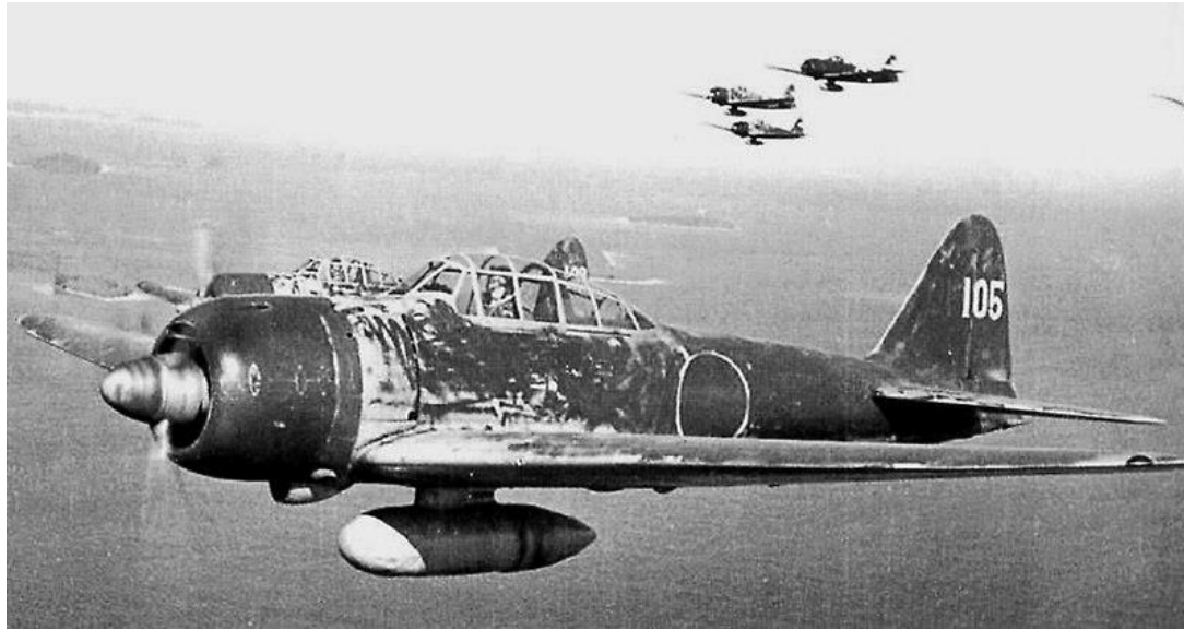
Navy A6M3 Model 22 (allied reporting name Zeke, colloquially Zero), over the Solomon Islands, 1943. 2 * 20mm cannon and 2 * .303 machine guns.
