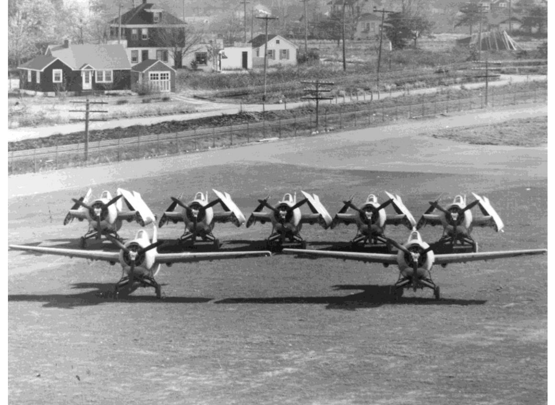
One of the main features of the F4F-4 were the Sto-Wing -design folding wings, a Grumman patented design.
