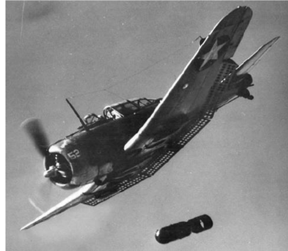
Douglas SBD (Scout Bomber) Dauntless Dive bomber Max speed 255 mph Strike radius 325 miles with 500 lb bomb load 250 miles with 1,000 lb bombload
