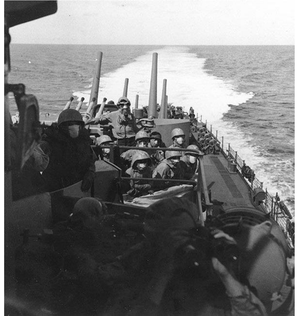
USS San Juan (CL 54) crew at general quarters at sea, circa 1942. Looking aft. 1.1" quadruple anti-aircraft machine gun mount in left center, 5"/38 guns beyond.
