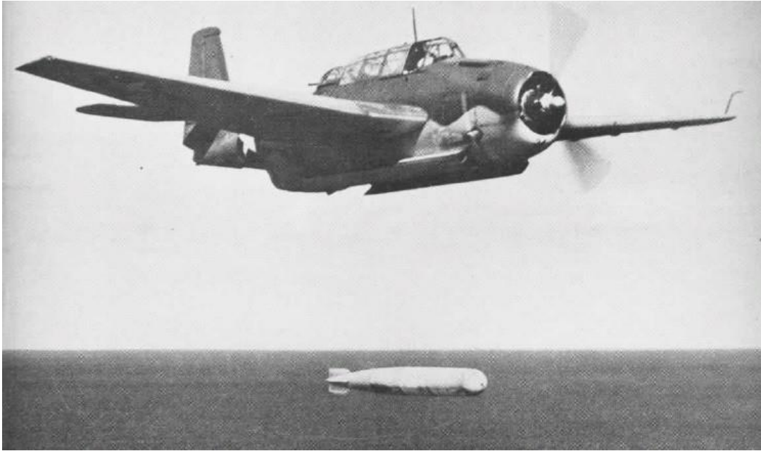
TBF Avenger dropping a torpedo Max speed 275 mph 1 torpedo or 2,000 lb bombs carried internally. Strike radius c 300 miles
