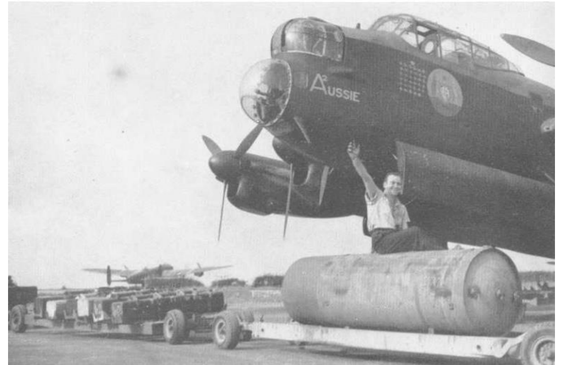
Preparing to bomb-up a Lancaster of No . 460 Squadron, armourer Cpl W. E. Dawson rides on a 4,000-lb high-capacity bomb (a "cookie"). while behind is a portion of the incendiary bomb containers which made up the normal load for area attacks. September 1943.
