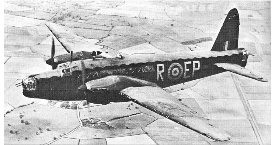
Merlin-engined Wellington Mark II of No. 104 Sqn. The criss-cross geodetic construction can be seen through the perspex panels in the side of the fuselage.
