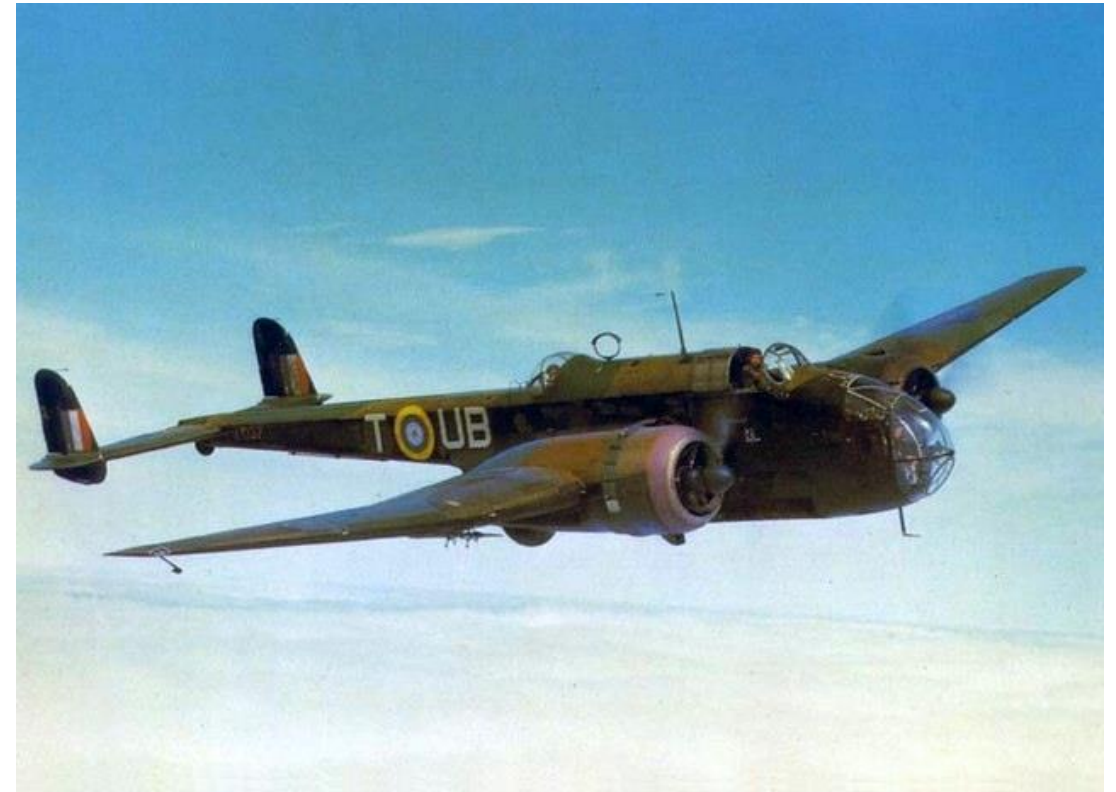
A Handley Page Hampden Mark I, AT137 'UB-T', of No. 455 Squadron RAAF based at Leuchars, Fife, Scotland (UK), in flight above clouds, May 1942. Max speed: 215 kn at 13,800 ft Cruise speed: 179 kn at 15,000 ft Range: 1,490 nmi with max fuel and 2,000 lb bombs. Service ceiling: 19,000 ft.
