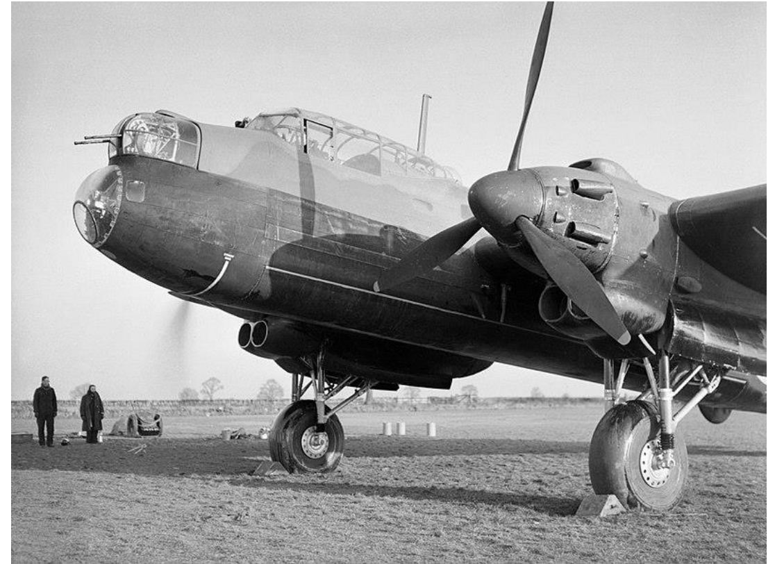
A Manchester Mark I showing the RR Vulture engine, which was the main cause of the design's failure. September 1941. The Vulture was an X24 42litre engine based on 2 V12 Peregrines joined by a new crank case and crankshaft.
