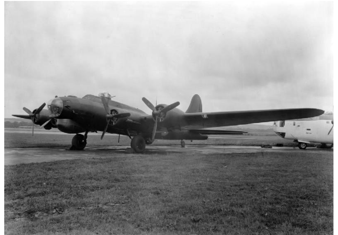
An electronic warfare Fortress III of 214 Squadron with nose-mounted H2S radome.
