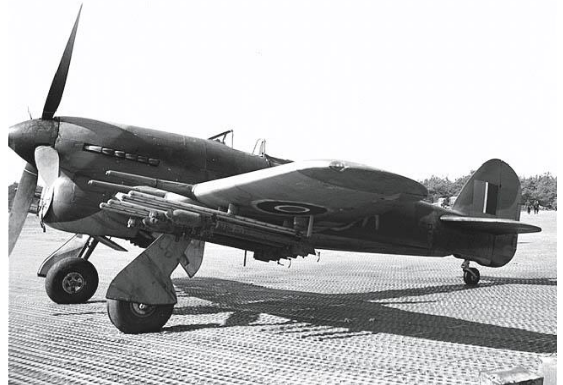
A late production Typhoon with full RP-3 armament, on the later aluminium Mk III rails, using a mix of SAP/HE 60 lb warheads (outermost rail and third) and the HE fragmentation head introduced in early December 1944 (2nd and 4th rail).
