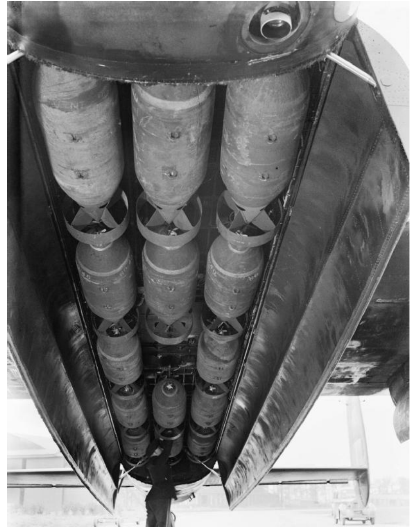
The bomb load used for industrial demolition (codeword 'Abnormal') in a Lancaster of No. 9 Squadron RAF, 1944. The "Usual" load consisted mainly of incendiaries.
