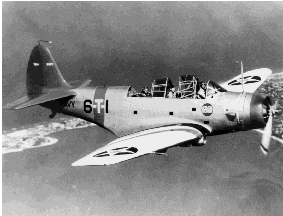
Douglas TBD-1 (Torpedo Bomber) Devastator of Torpedo Squadron Six (VT-6) Max speed 206 mph but limited to 110 knots for torpedo dropping
