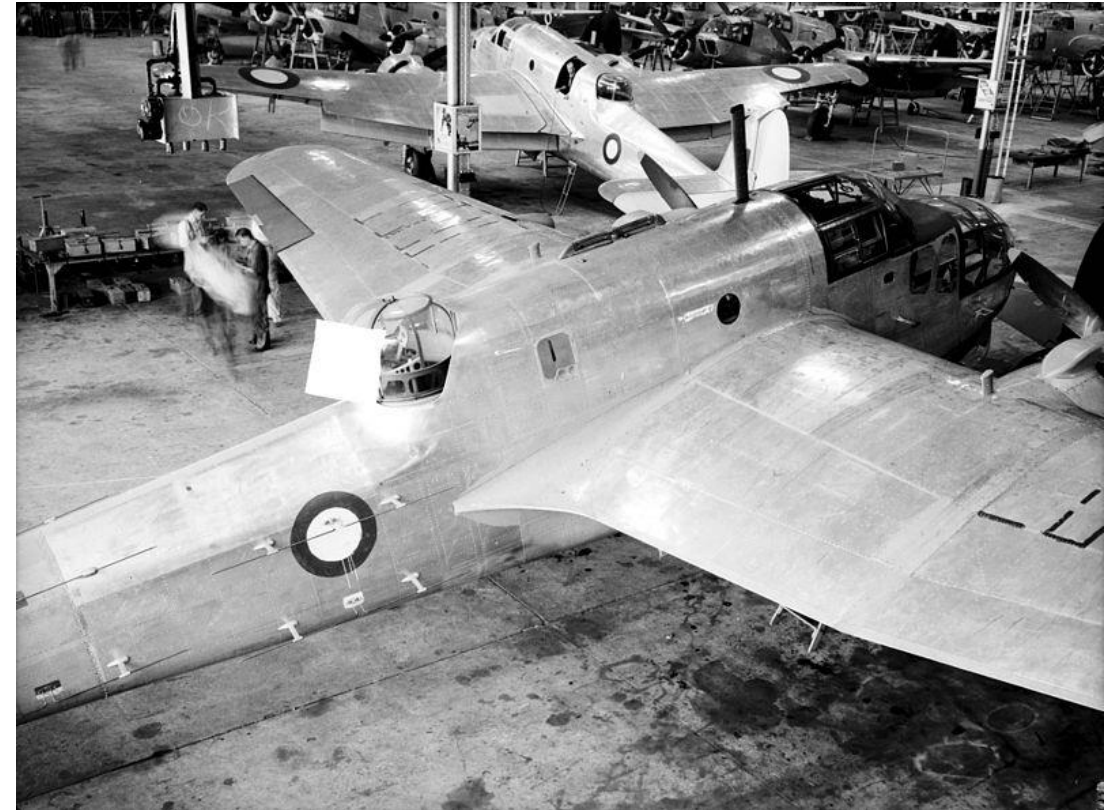
Beauforts being built at the DAP plant in Fishermans Bend, Melbourne. The ASV radar aerial array on the rear fuselage and a small blue/white Pacific Theatre roundel indicates this is a late Beaufort Mk VIII.
