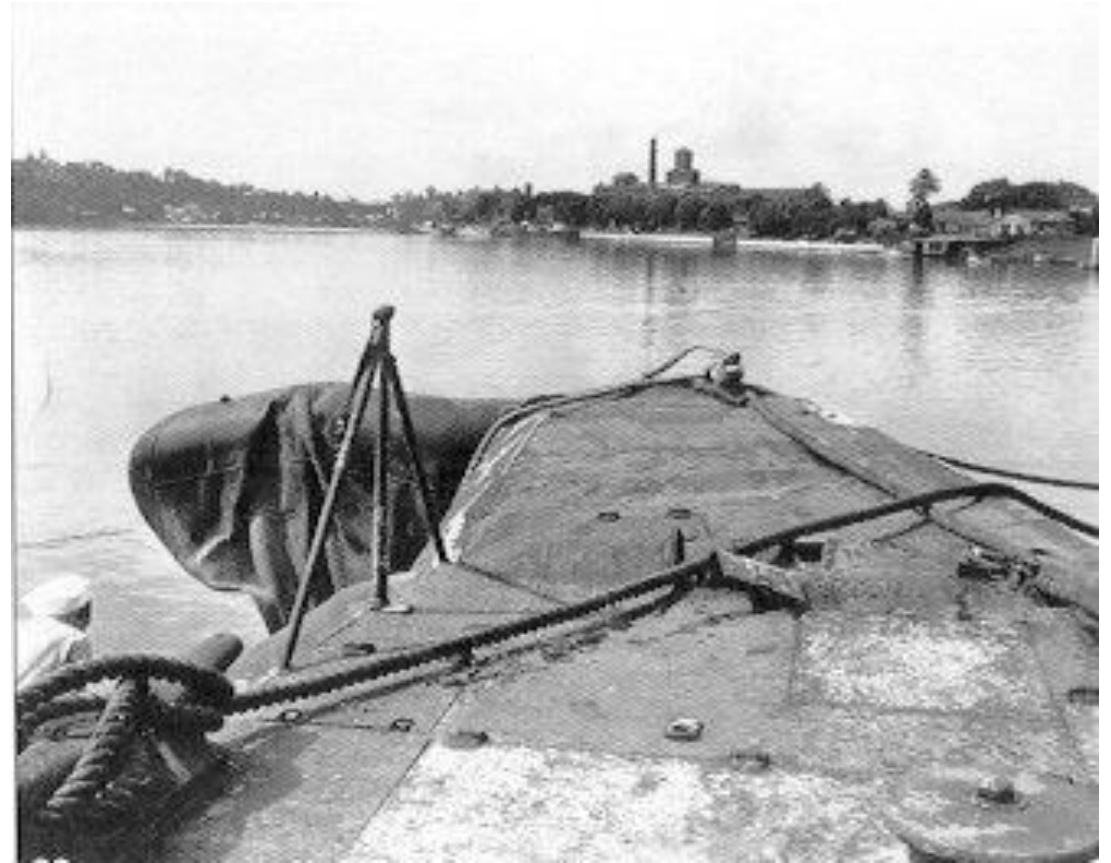
Growler's bent bow before repairs in Brisbane.
