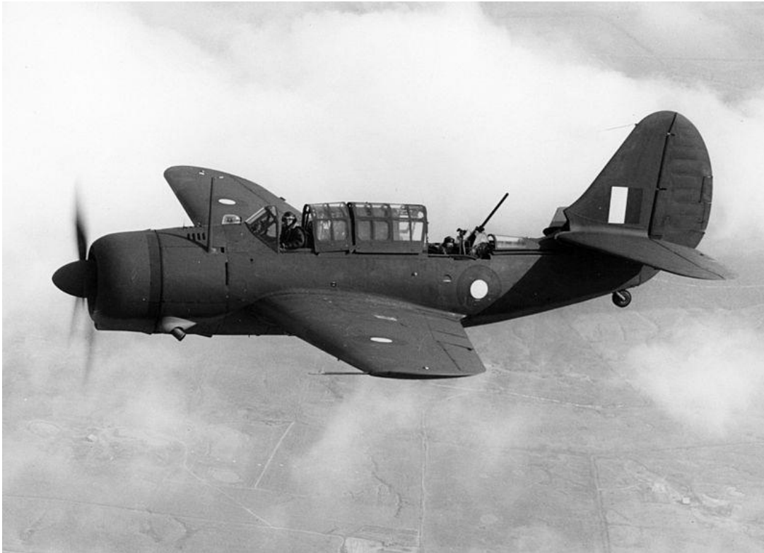
A69-4, the only Curtiss Shrike to enter RAAF service. It is an army version of the navy's SB2C Helldiver.
