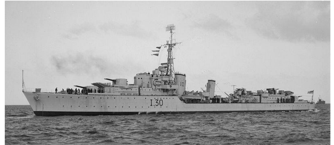
HMAS Arunta, tribal class destroyer. Builder Cockatoo Docks and Engineering Company. Laid down 15 November 1939, Launched 30 November 1940, Commissioned 30 March 1942. 2,000 tons, 36 Knots, 6 4.7 inch guns. Warramunga was a sister ship by the same builder on a similar time frame.
