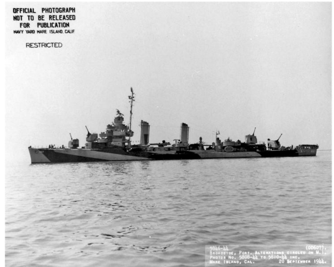
USS Frazier (DD-607), a Benson-class destroyer, 1,620 tons, 37.5 knots, 4 * 5 inch guns. Commissioned 30 July 1942.
