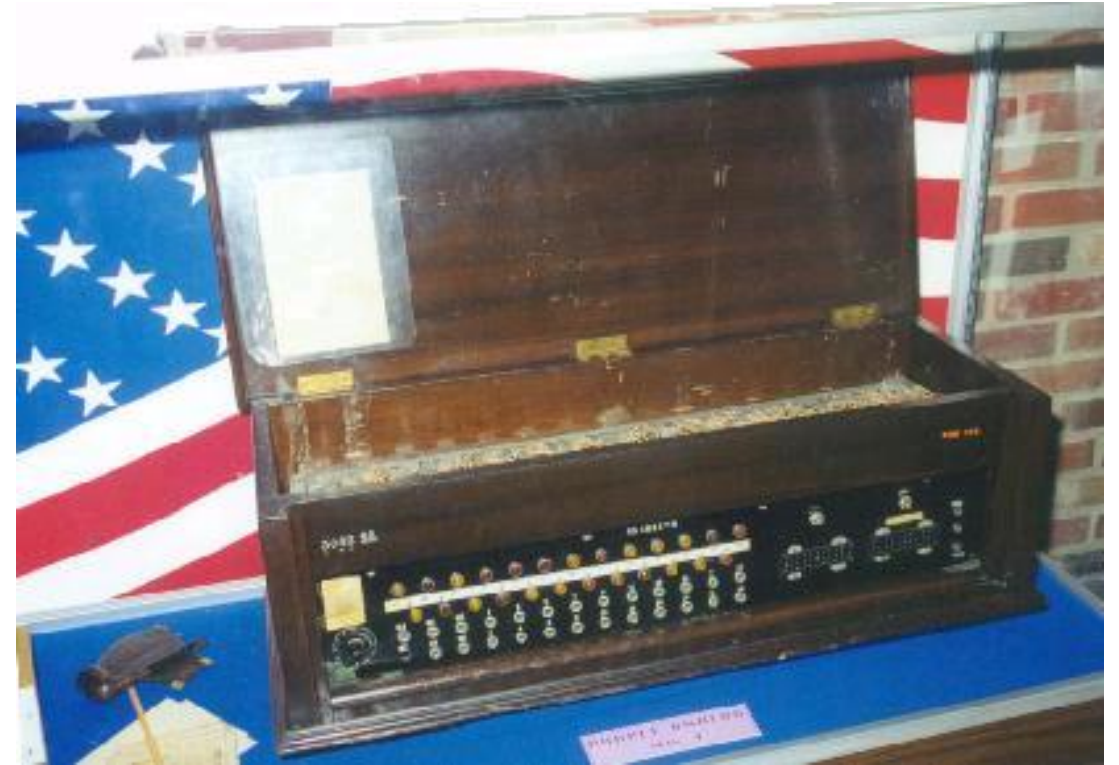
US functional replica of the Japanese Diplomatic Purple cipher.
