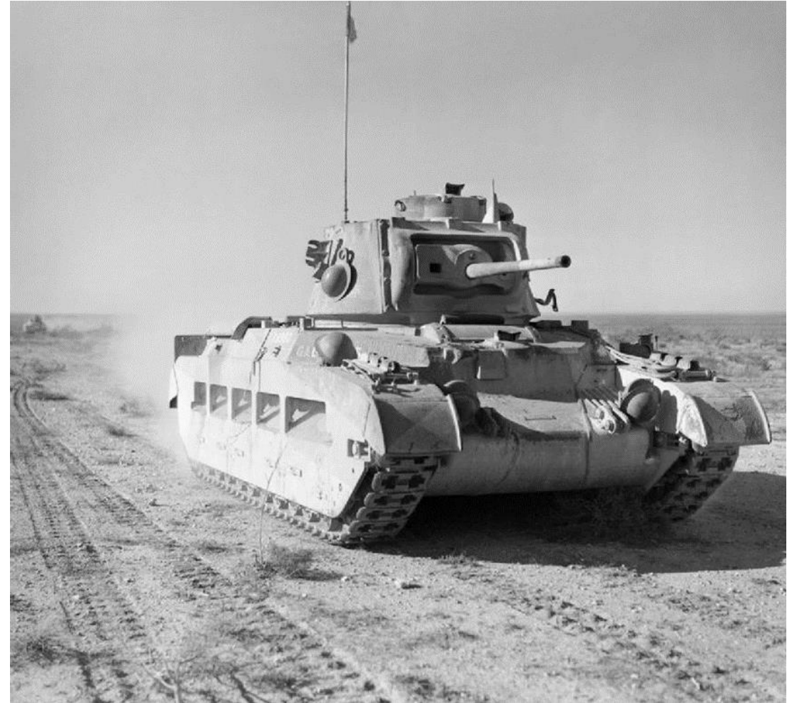
A Matilda 2 Infantry Tank. 25 tons, crew of four, 2 pounder gun, max speed 16mph on road, 9 mph off road.
