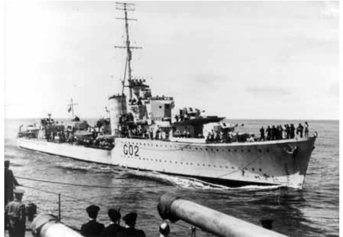
HMAS Nestor, 36 knots, 6 4.7 inch guns, 1 4inch AA gun, 10 torpedo tubes and depth charges.
