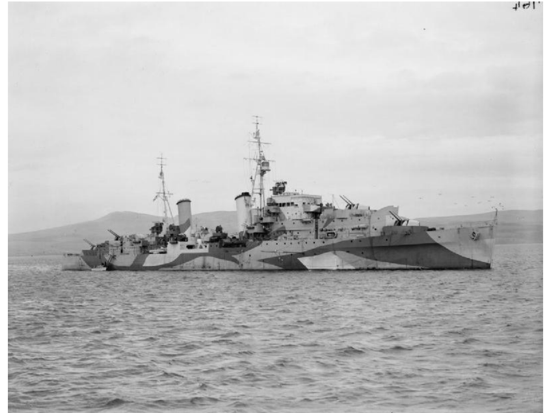
Anti-aircraft cruiser HMS Scylla. Her four twin 4.5-inch gun mountings are controlled by the two High Angle Director Towers, one sited behind the bridge and the other abaft the after funnel.
