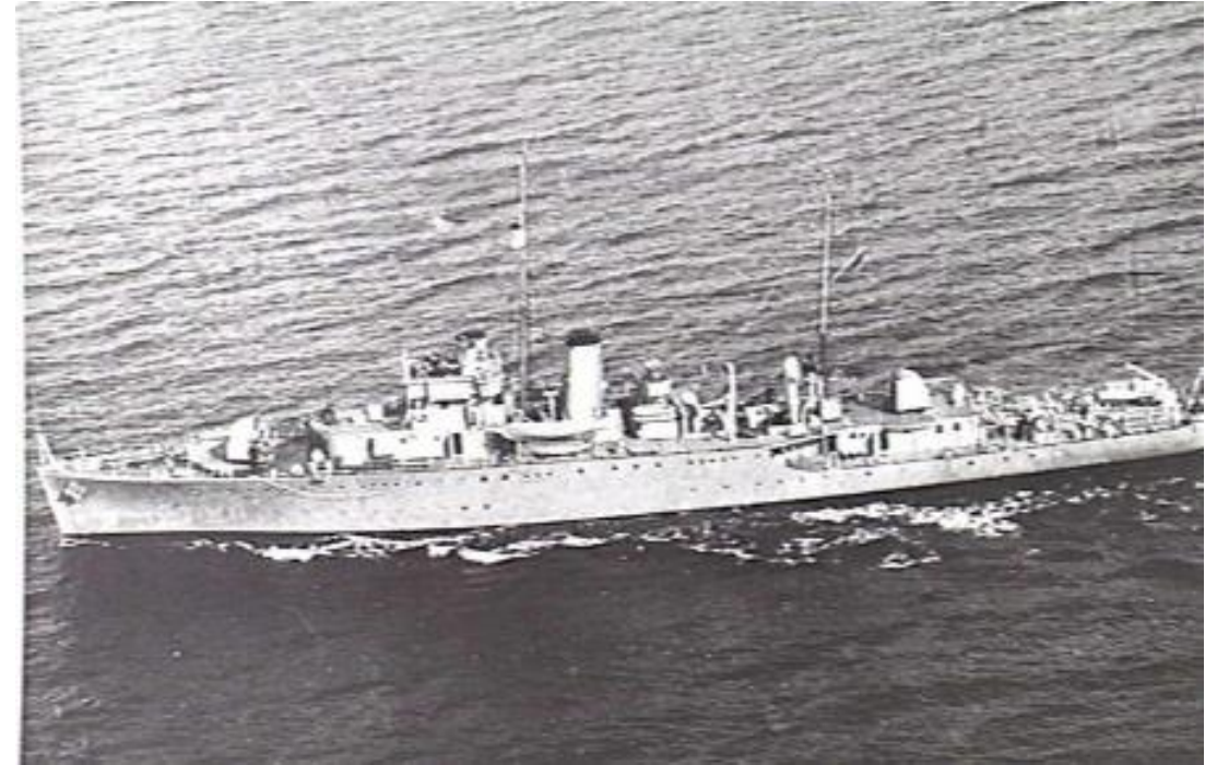
HMAS PARRAMATTA (II). NOTE THE 4 INCH MARK XVI GUNS IN A TWIN MARK XIX MOUNTING FORWARD AND A SINGLE MARK XX AFT. A QUADRUPLE .5 INCH AA MACHINE GUN IS MOUNTED IN B POSITION. FIRE CONTROL WAS PROVIDED THE HIGH ANGLE CONTROL SYSTEM SITED BEHIND THE BRIDGE. NOTE THE KITE/OTTERS AND FLOATS OF THE OROPESA MINESWEEPING GEAR ON THE QUARTERDECK."
