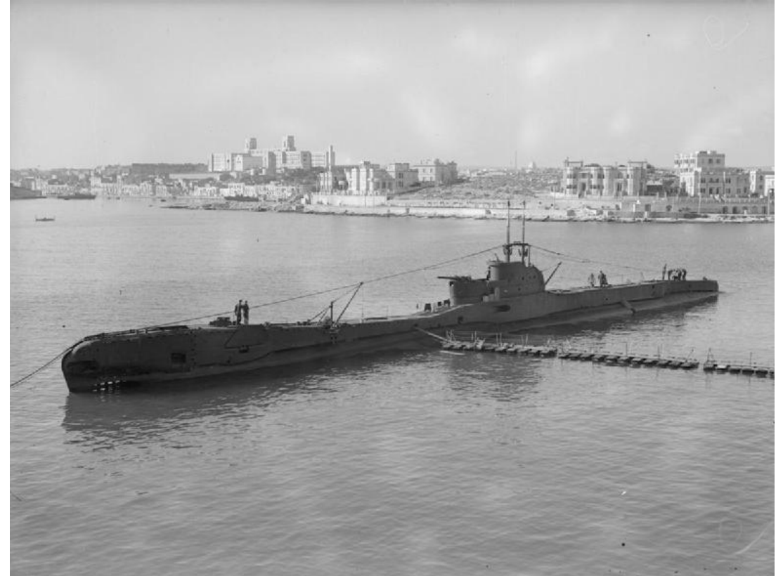
HM Submarine Taku, 1,090 tons surfaced, 1,575 tons submerged. Length 275 ft, Six internal forward-facing 21 inch torpedo tubes, Four external forward-facing torpedo tubes, Six reload torpedoes, One 4-inch gun.
