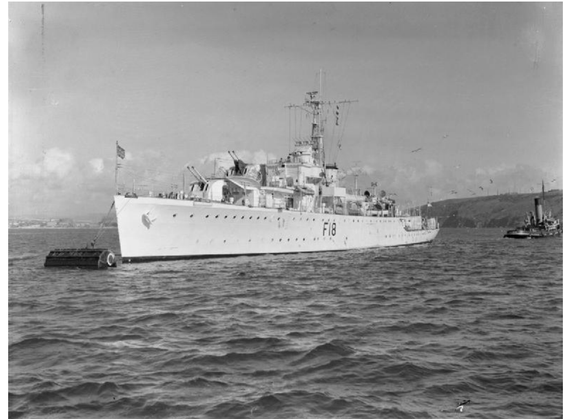
HMS Flamingo, a Black Swan-class sloop, 1,350 tons, 19 knots, 6 4inch guns.
