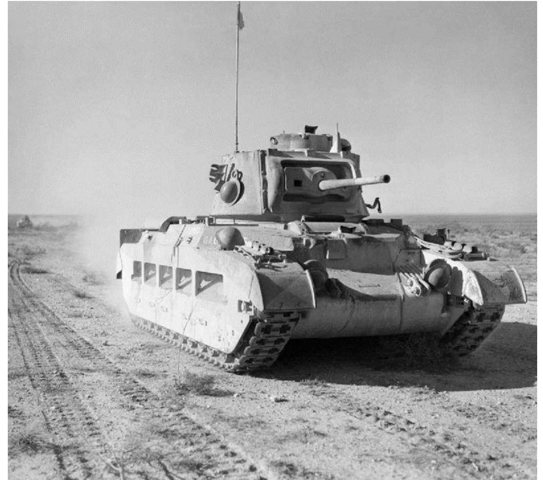
A Matilda 2 Infantry Tank. 25 tons, crew of four, 2 pounder gun, max speed 16mph on road, 9 mph off road.
