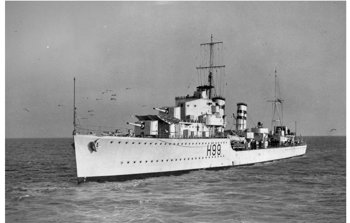
HMS Hero. 1,350 tons 36 knots 4 4.7 inch guns, 8 21 inch torpedo tubes.
