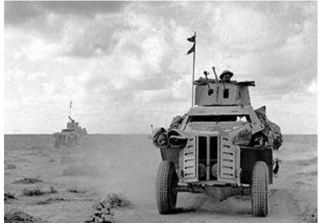
Marmon-Herrington armoured cars on patrol in the Western Desert, 28 November 1941. Mark II, "Middle East Model" denoted the vehicles serving with British forces in the North African campaign. This variant was fitted with a Boys anti-tank rifle and a single coaxial Bren light machine gun.
