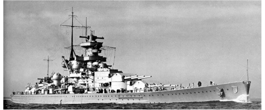
The battleship Scharnhorst. She and her sister ship Gneisenau had 9 eleven inch guns a max speed of 31 knots and a 14 inch thick armor belt.
