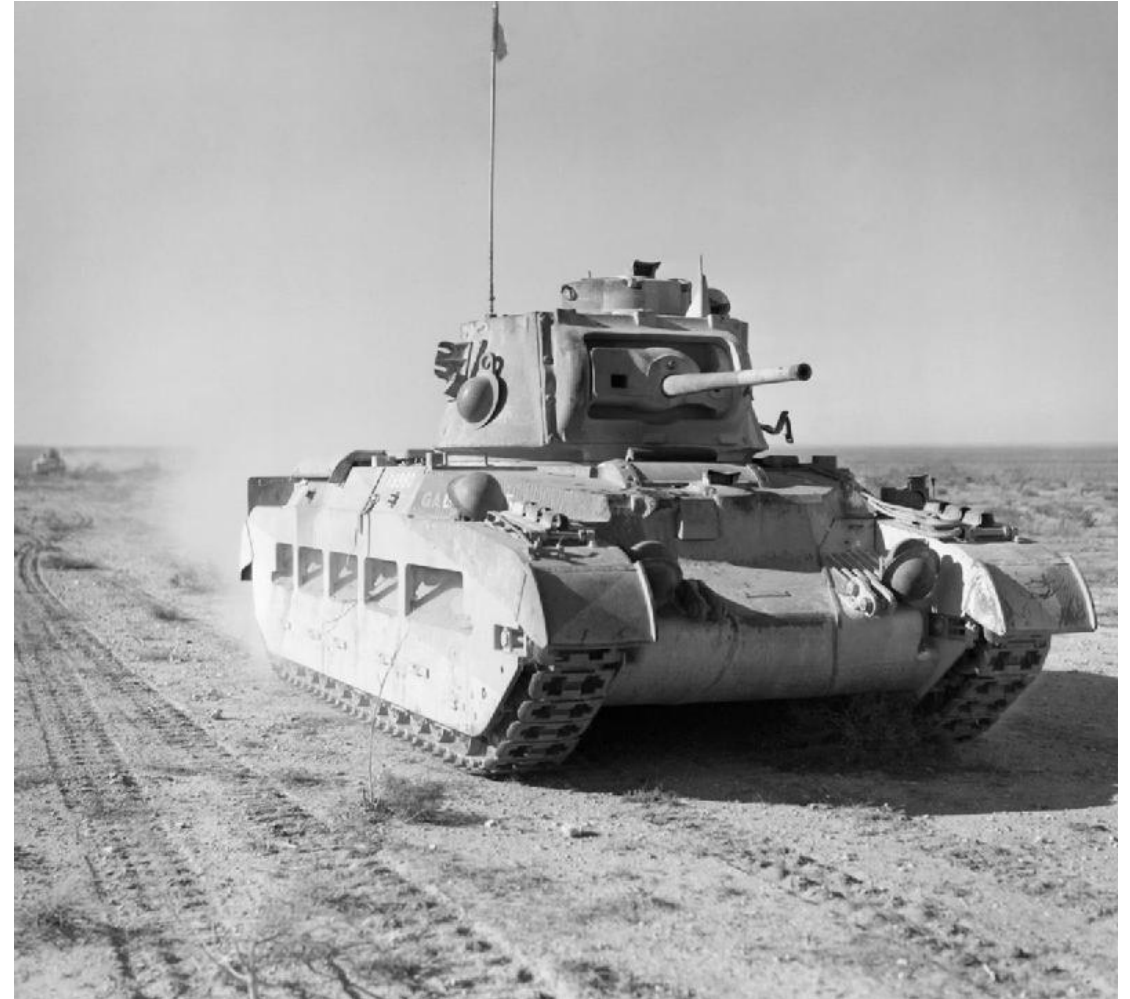
A Matilda 2 tank of the 7th Royal Tank Regiment. 25 tons, crew of four, 2 pounder gun, max speed 16mph on road, 9 mph off road.
